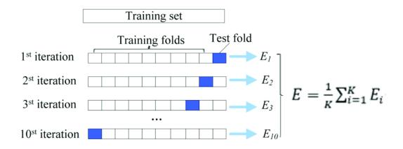
Figure 4.2. How the cross validation work
