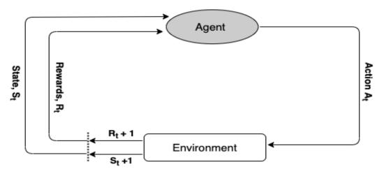
Figure 5.1: Reinforcement learning process
