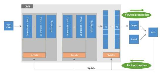
In CNN final classification layer takes the output of the final convolution layer as input and higher convolution layers detect complex objects.
